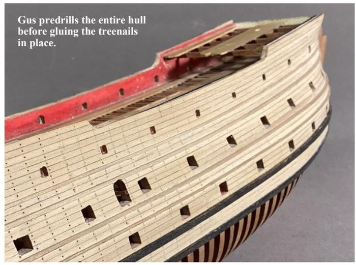
Gus predrills the entire hull before gluing the treenails in place.
