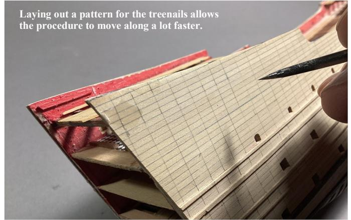
Laying out a pattern for the treenails allows the procedure to move along a lot faster.
